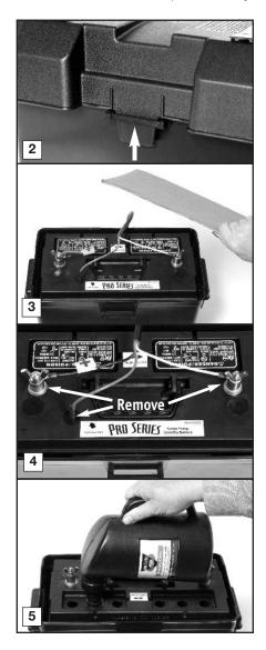
The hole is marked with an arrow. Replace the battery cables...the WHITE wire to the NEGATIVE (-) post, and the BLACK wire to the POSITIVE (+) post. Replace the wing nuts and tighten.
