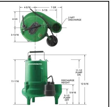
All dimensions in inches. Metric for international use. Component dimensions may vary  $\pm$  1/8 inch. Dimensional data not for construction purpose unless certified. Dimensions and weights are approximate. On/Off level adjustable. We reserve the right to make revisions to our product and their specifications without notice.
